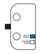
If the switch is configured for monitored reset, the last switch will indicate the status of the reset circuit / external device with a blue LED. Once the system has been reset, the blue LED will turn OFF.
