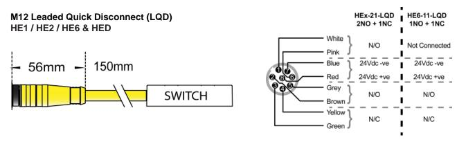
**CONTACT OPERATION** -The N/O contact(s) on Mechan safety switches are open when the actuator is away from the switch. When the actuator is within the specified operating distance the N/O contact(s) will close and the N/C contact will open
