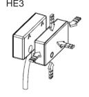
The HED double switch is designed to monitor two adjacent doors.
