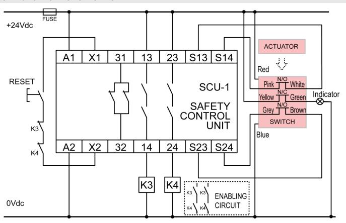
NOTE 1 : THE SCU-1 SAFETY CONTROL UNIT IS DESIGNED TO WORK WITH 2 X NO INPUT FROM THE HE SAFETY SWITCHES
