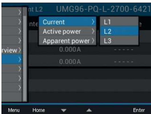
Fig. Drag indicator display with the submenu items Current , Active power and Apparent power .
