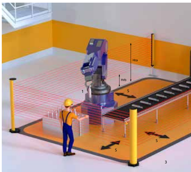
Fig. 38. Scenario 3 - Possibility to reach the hazardous point by leaning against the mechanical protection and bypass the light curtain
