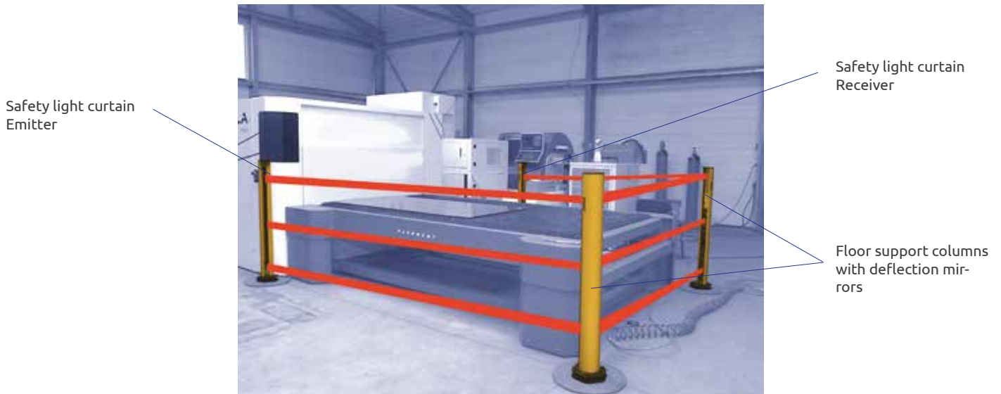
Fig. 47. Machine for laser cutting perimeter protection
