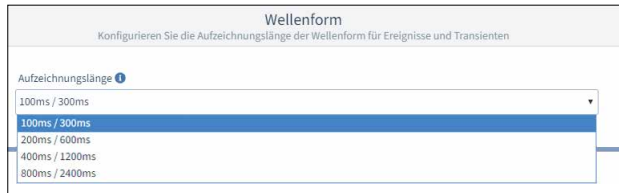
Fig. Waveform window with the configuration of the lead time and lag time in the Recording menu of the GridVis software - Configuration of the recording length.
