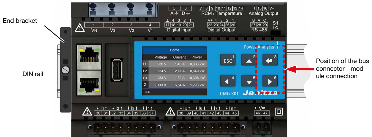
Fig. 5: Device with terminals on DIN rail according to DIN EN 60715 (front view)
