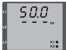
Fig. No rotation field direction detectable.
