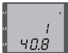
Fig. Operating hours meter of the measured value display The UMG 96RM-P/-CBM shows the number 140.8h in the operating hours meter. This corresponds to 140 hours and 80 industrial minutes. 100 industrial minutes correspond to 60 minutes. In this example, 80 industrial minutes therefore represent 48 minutes.
