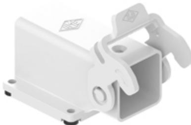
Angled Bulkhead mounting housing, CK series, with 1 lever without cable entry, size "21.21", fixing by 4 screws
