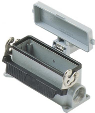
Surface mounting housing, C-TYPE series, with 1 lever, M32 x 2 cable entry, size "104.27", high construction, with plastic cover
